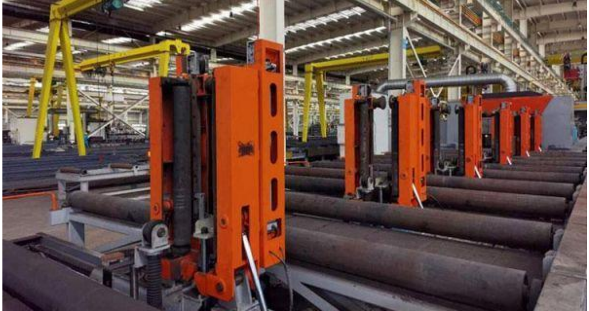
Device to lift the web and flip up the flanges
